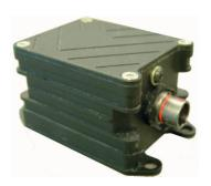
The PSU30V serves to boost and stabilise the car supply voltage from 14V nominal to 30V stabilised. This is to enable actuators to be driven from a regulated 30V supply instead of the unregulated 14V car supply. For solenoids, this allows faster actuation times.
